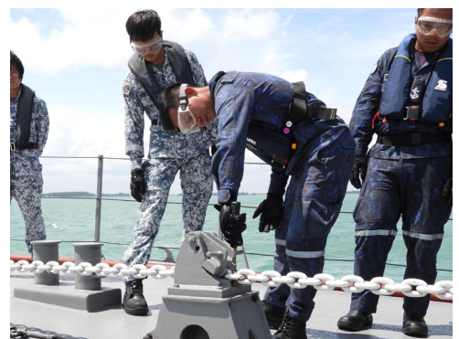
AB Pg Hafiz operating the devil's claw (chain stopper).
